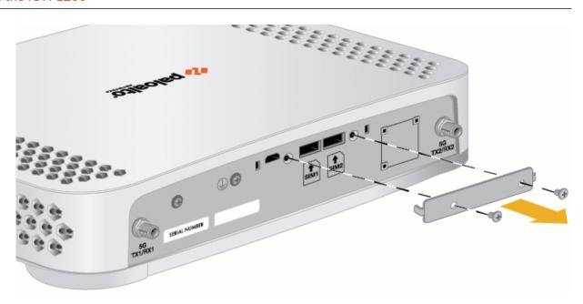
**STEP 3** After inserting the SIM, place the SIM cover back on the device.
