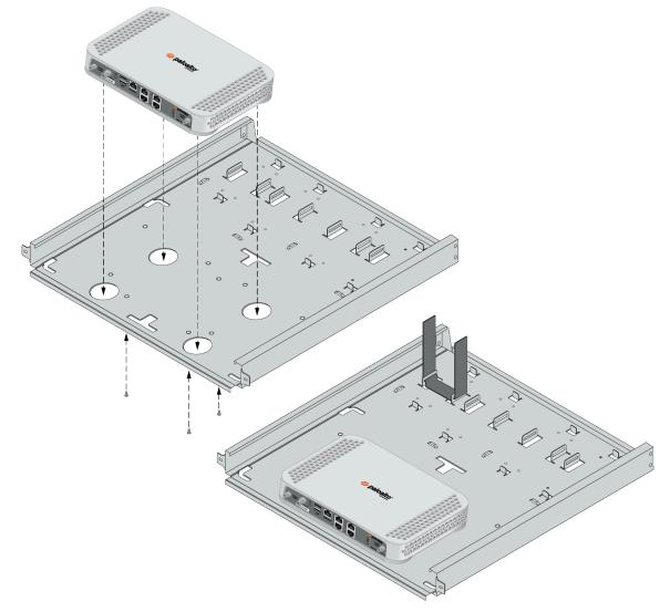
**STEP 5** | Secure the device in place using three of the provided #6-32 x 3/16" Long Flathead screws.
