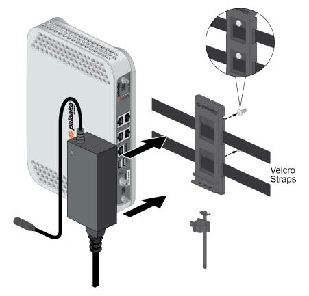
The following image shows a completed installation for an ION 1200 with a single power adapter.
