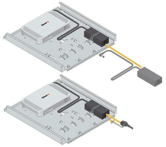
**STEP 7** | Plug the power supply connector into the back of the device. Using the provided tie-wraps, bind and secure the power supply cable to the metal hooks in the mounting tray.
