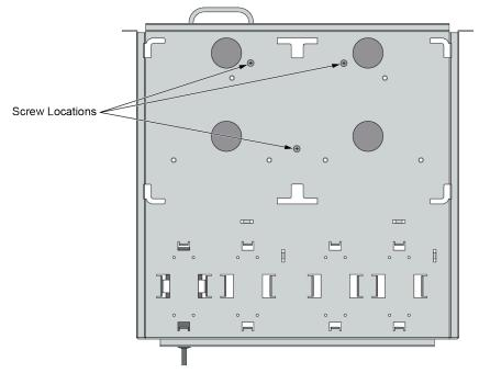
**STEP 6** | Slide the device power supply into the marked position and fasten the provided velcro strap around the power supply until it is secure in place.
