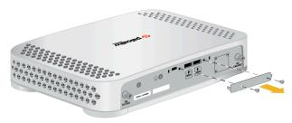
**STEP 2** Insert the nano SIM in SIM 1 or SIM 2 slot by pushing the SIM in the slot till it is locked in its position.
