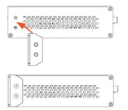
**STEP 3** Attach the L-shaped brackets to the screw holes on either the front or back of the device.
