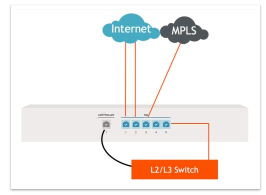
**STEP 5** Connect the cables for controller, internet, and LAN or WAN ports.
