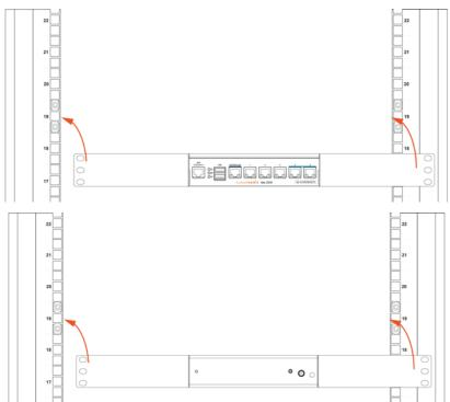
**STEP 6** | Finally, verify that the device is securely mounted on the rack.
