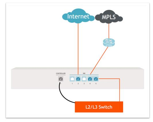
**STEP 5** Connect the cables to controller, internet, and LAN or WAN ports.
