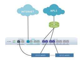
• Dual Router or Dual Switch—The following image illustrates the deployment architecture of an ION 3000 as dual router or dual switch.
