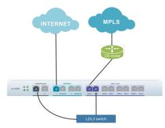
• Single Router or Dual Switch—The following image illustrates the deployment architecture of an ION 3000 as single router or dual switch.
