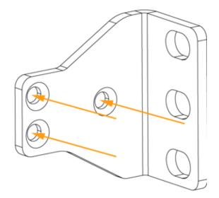
After you attach the ears, mount the ION 3000 to any standard 19 inch rack using three appropriate screws for the specific 19 inch rack.
