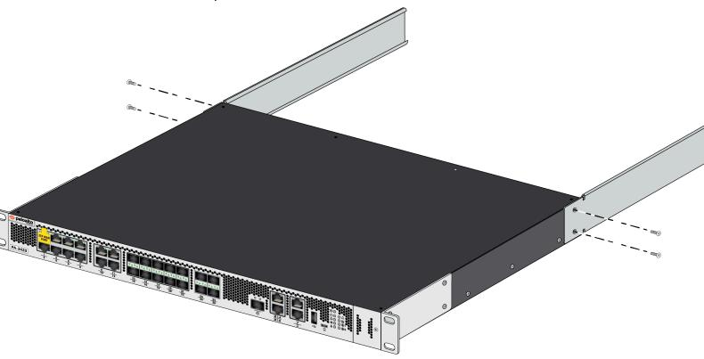
STEP 3 | With help from another person, hold the firewall in the rack and secure the front rack-mount brackets to the front rack-posts using two screws for each bracket. Use the appropriate
