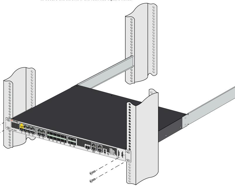
STEP 4 | Slide one back rack-mount bracket into each of the two previously installed side rack-mount rails and secure the brackets to the back rack-posts using the appropriate screws for your rack (#10-32 x 3/4" or #12-24 x 1/2") and torque to 25 in-lbs.
