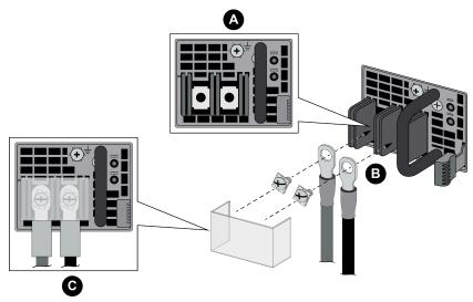
STEP 4 After all DC power cables are securely connected, power on the DC power sources. The power supplies powers on, the input and output LEDs on the power supplies turn green, and the PWR LED and the power supply LEDs (PWR 1 and PWR 2) on the front of the firewall turns green.
