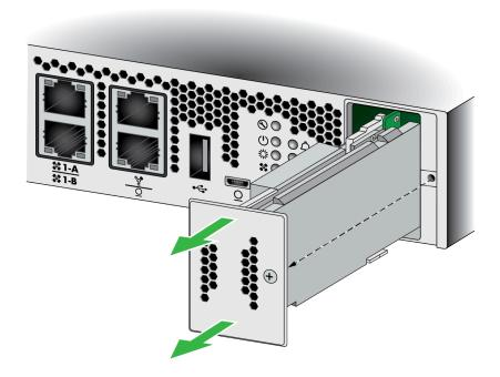
STEP 4 | Slide the replacement SSD module onto the rails and gently push it into the firewall.
