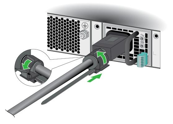
STEP 5 | Connect the other end of the power cords to an AC power source. After the power supply is connected, the power supply powers on, the input and output LEDs on the power supply turn green, and the PWR LED and the power supply LED (PWR 1 or PWR 2) on the front of the firewall turns green.
