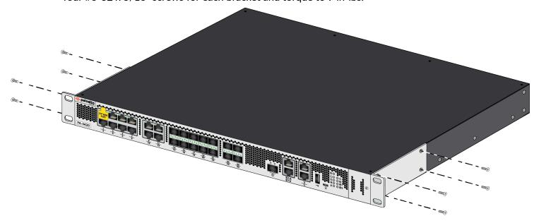
STEP 2 | Attach one rack-mount rail to each side of the firewall using two #6-32 x 5/16" screws for each rail and torque to 9 in-lbs.
