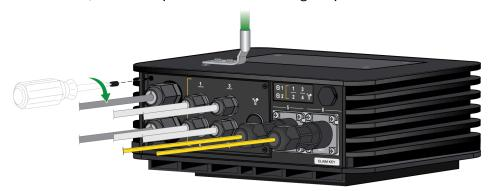
3. Push the end caps along each Ethernet and power cable until the end caps reach their respective panel connector. Screw the end caps onto each panel connector, making sure that it is tight and secure.
