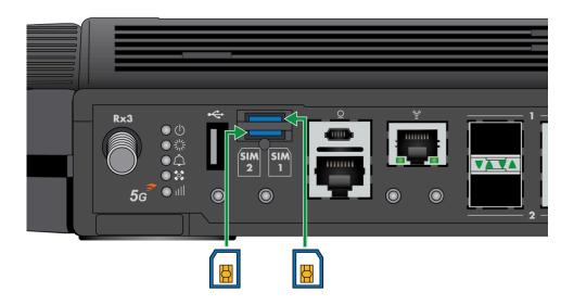
STEP 3 | After inserting the SIM, place the SIM cover back onto the device and refasten the screw(s).
