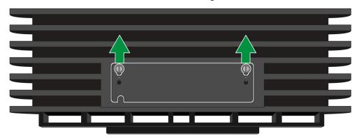
PA-450R-5G—Unfasten the two screws using a Philips head screwdriver.
