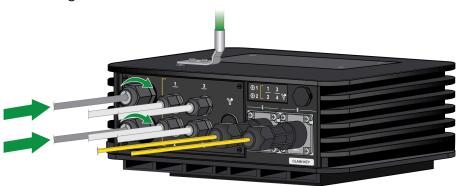
STEP 9 | Power on the DC power source to power on the firewall. The firewall powers on and the power LED turns green.
