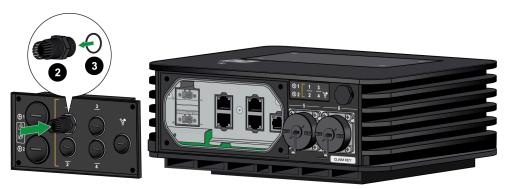
STEP 5 | Thread the cable through the end cap. This is used to secure the cable gland once the panel is reattached at the end of the procedure. Feed the cable through the gray grommet. Move the cable through the panel connector and gently push the end into the port until you hear a click.
